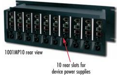
The Model 1001MP series offers a convenient method for converting your favorite Patton standalone product into a rack-mounted solution.
